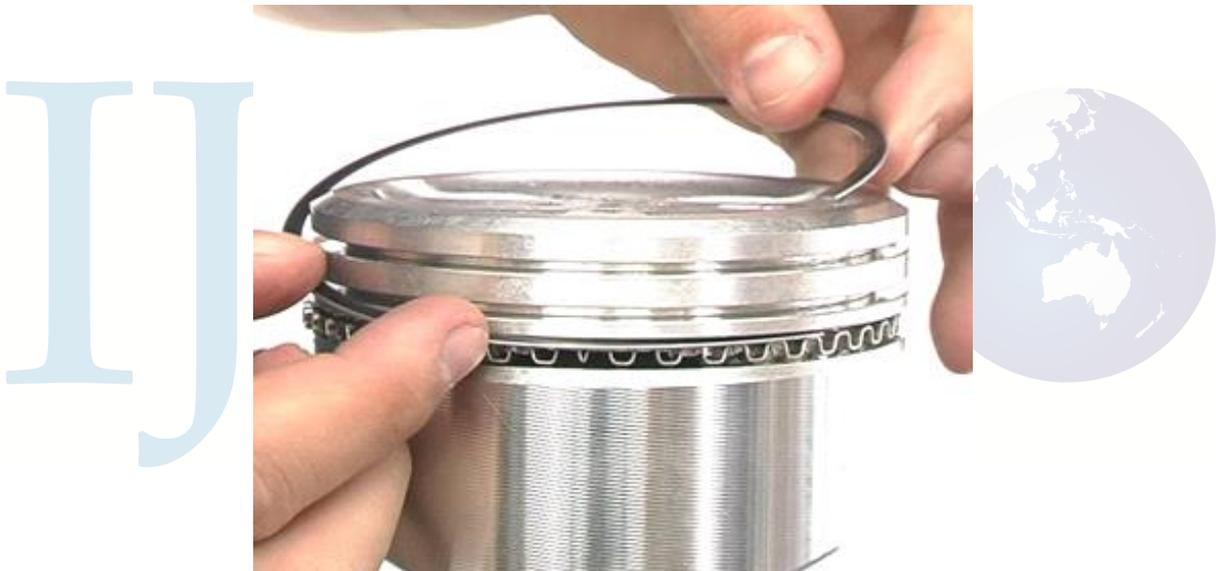
The last ring is called the **oil ring**. These work with the piston in the engine to lubricate the cylinder, walls, pistons, rings, and wrist pins. This ring keeps the oil out of the combustion process. The oil rings also help the thermal control because it cools the piston by directing oil around it. The piston rings are located on the piston. The [piston](#) is located in the cylinder, and multiple cylinders are usually arranged side by side in a bank. This bank is known as the engine block.
