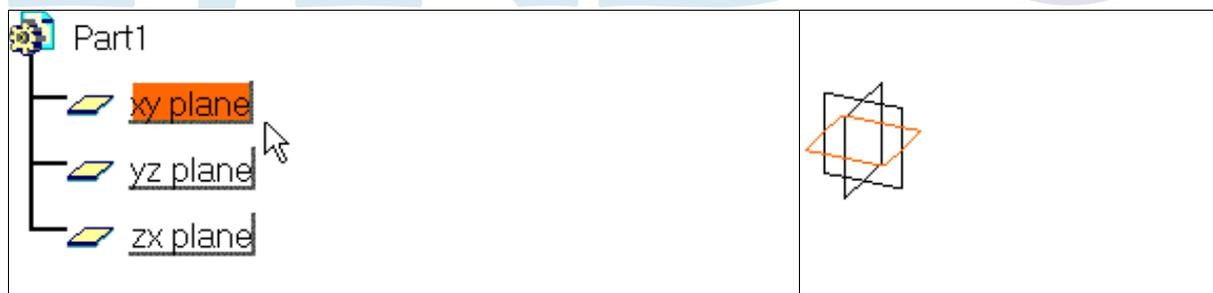
Select one plane of the local axis. h and v are aligned to the main axes of this selected plane. Associativity is kept between both the plane and the sketch.
