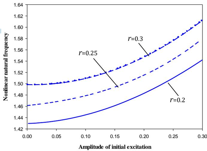
Fig. 6. Effect of r ratio on nonlinear natural frequency.
