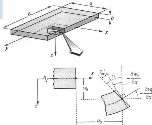
Fig. 1. Rectangular isotropic plate and its displacement after deflection.
