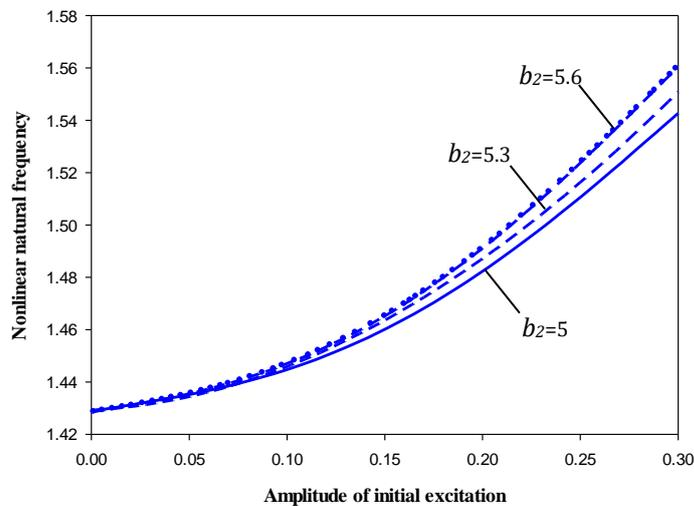
Fig. 7. Effect of nonlinear factor  $b_2$  on nonlinear frequency.
