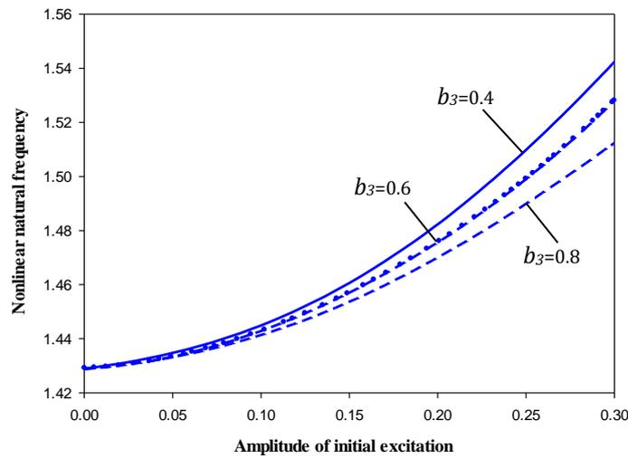
Fig. 8. Effect of nonlinear factor  $b_3$  on nonlinear frequency.
