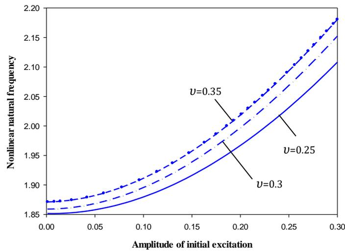
Fig. 5. Effect of Poisson's ratio on nonlinear frequency.
