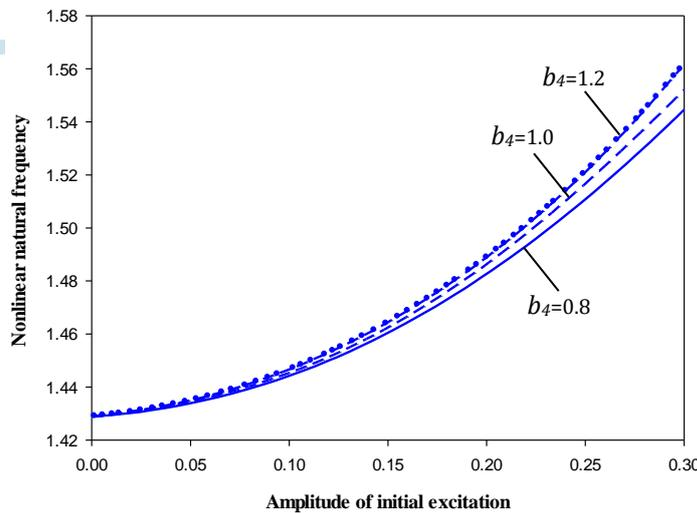
Fig. 9. Effect of nonlinear factor  $b_4$  on nonlinear frequency.
