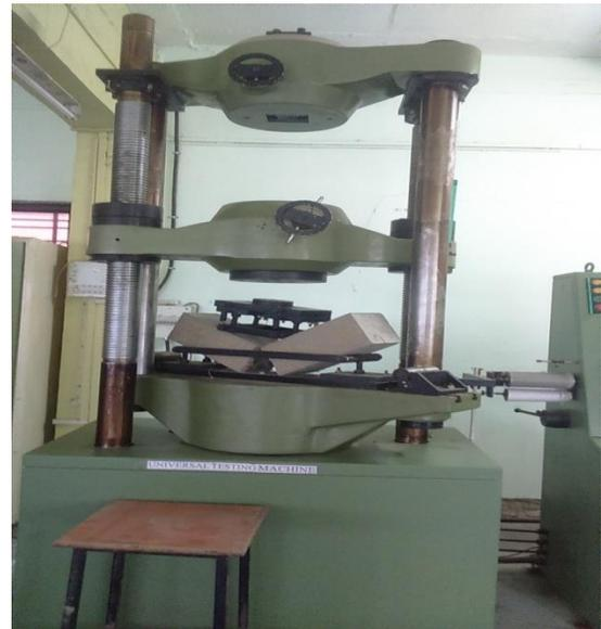
Testing Of Concrete Beam Specimen
