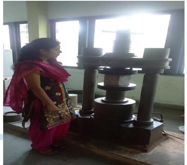
Testing of Concrete Cube Specimen
