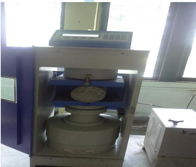
Testing Of Concrete Cylinder Specimen
