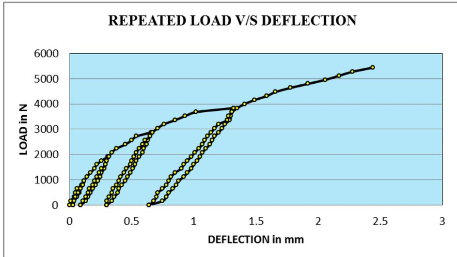
Fig 6: Repeated load V/s Deflection Diagram for 2 Layers of Mesh and 10% Replacement of BFS Slag
