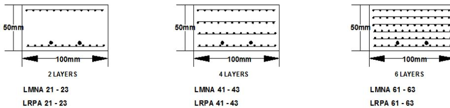
**GROUP A :- UNIFORMLY SPACED WITH 4mm M.S.BARS ON TENSION SIDE**
