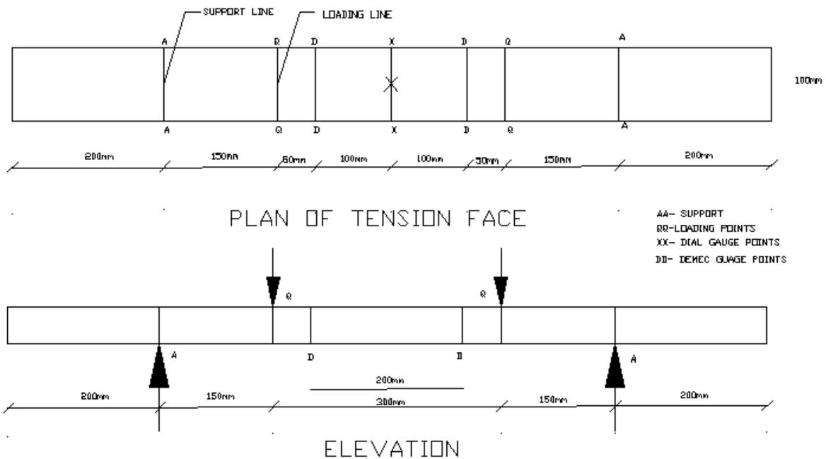
Details of Demec & Dial Gauge Points specimens
