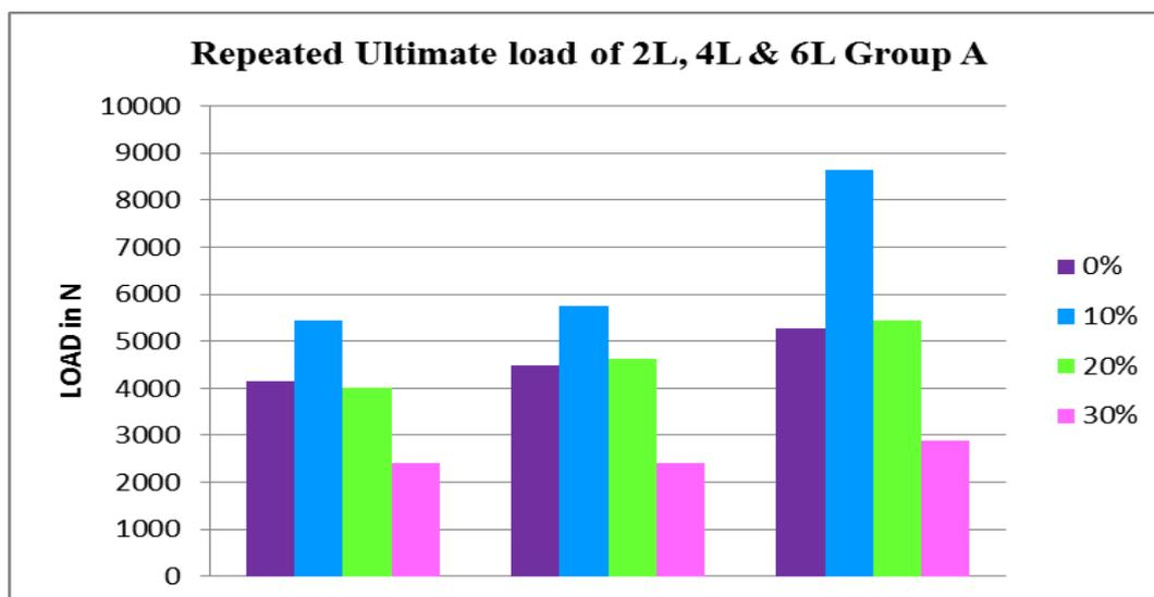
**Fig 8: Repeated Ultimate load Diagram for 2, 4, 6 Layers of Mesh and 0%, 10%, 20% & 30% Replacement of BFS Slag Respectively .**
