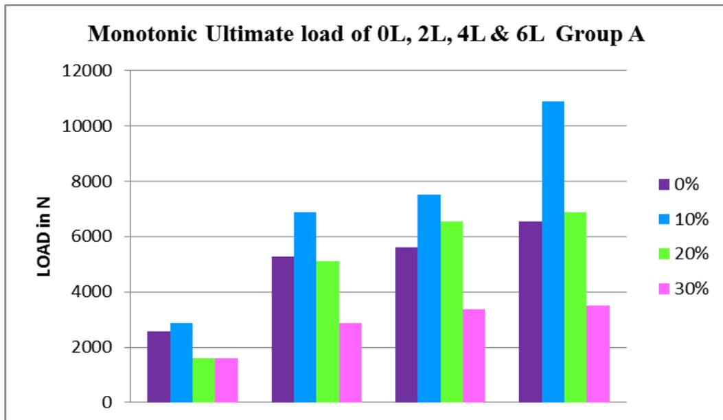
Fig 7: Monotonic Ultimate load Diagram for 0, 2, 4, 6 Layers of Mesh and 0%, 10%, 20% & 30% Replacement of BFS Slag Respectively
