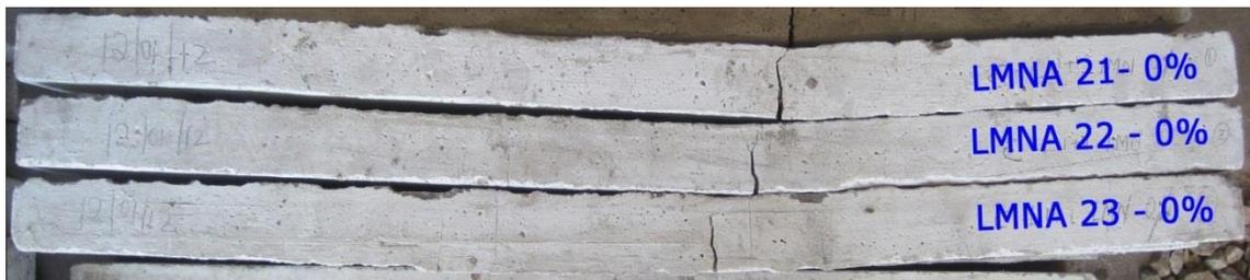
**Fig4 – Failure of 2L Specimen in 0% Replacement of B.F.S under Monotonic Loading**
