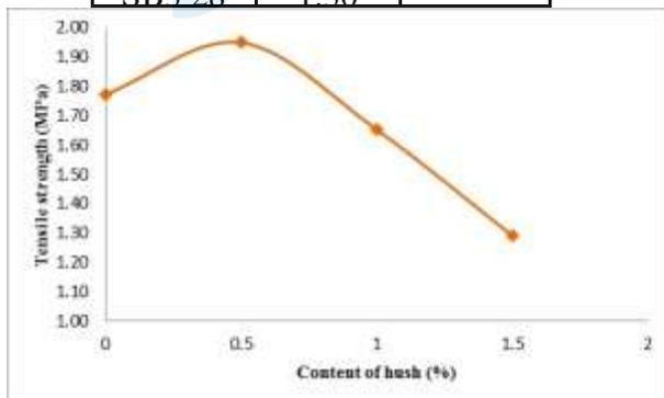
Figure 6. curve of hush content with split strength
