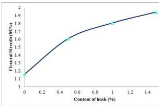
Figure 7. curve of hush content with flexural strength
