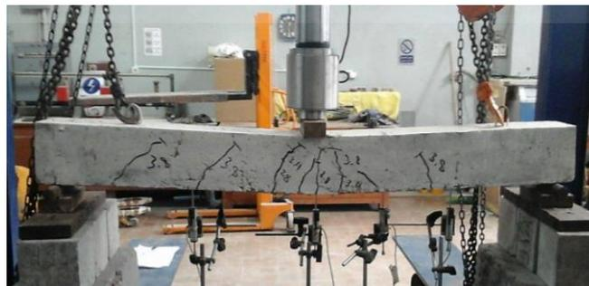
Fig. 7 Typical reference beam failure mode.
