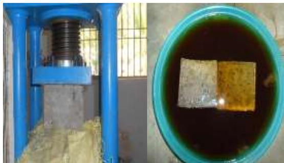
**Figure 2 Compressive test and Immersed in Acid and Chloride solution**
