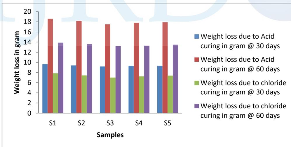
**Figure 3 Weight loss due to Acid and Chloride curing @ 30 and 60 days**
