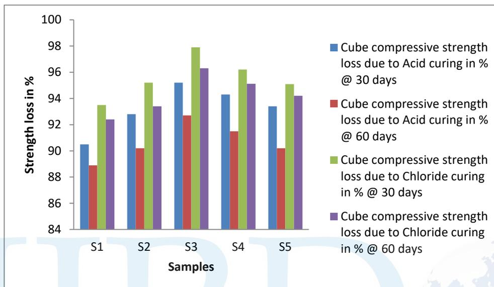
**Figure 4 Cube compressive strength loss due to Acid and Chloride curing @ 30 and 60 days**
