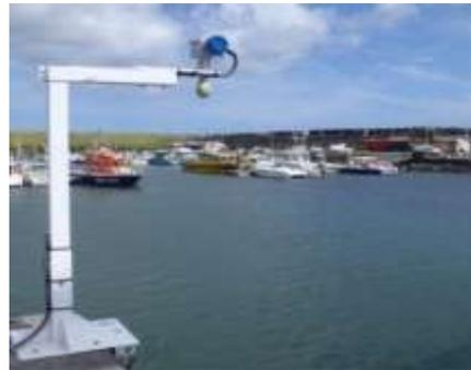
**Figure (2):** shows the proposed radar gauge station [12].
