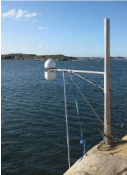
**Figure (4):** the antenna closed to the tide gauge hut [14][28]
