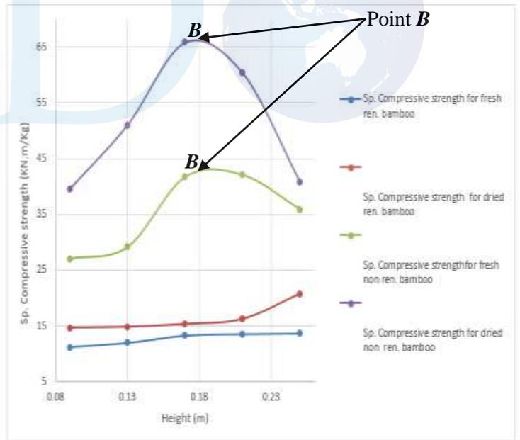
Fig. 4.0 Specific Compressive Strength VS Height
