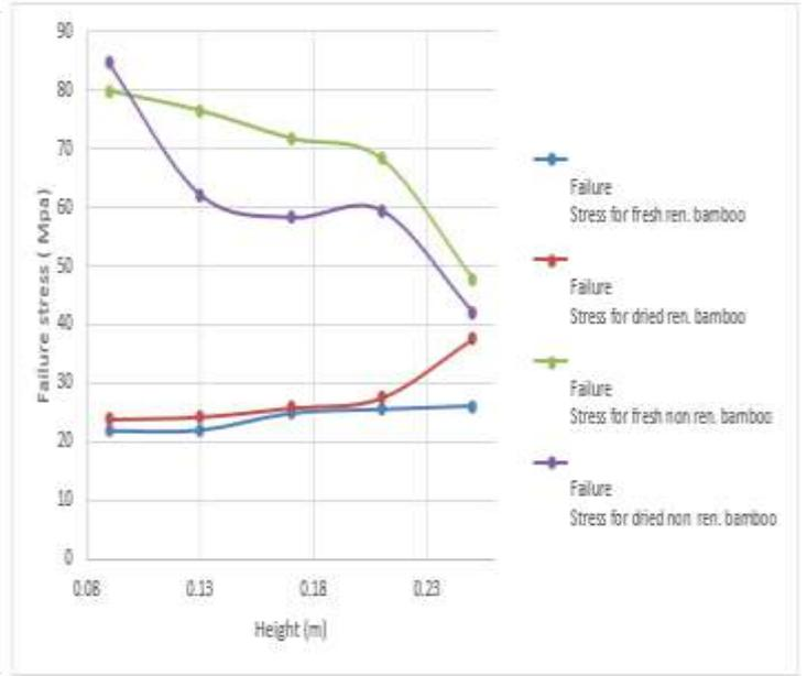
Fig. 3.6 Failure Stress VS Height
