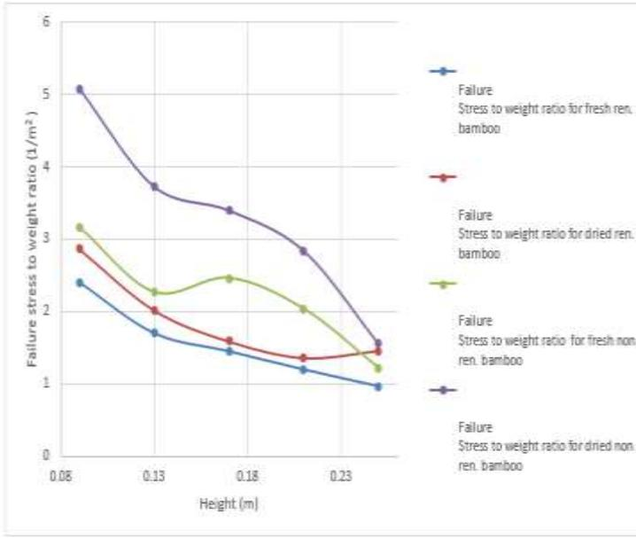
Fig. 3.5 Failure Stress to Weight Ratio VS Height
