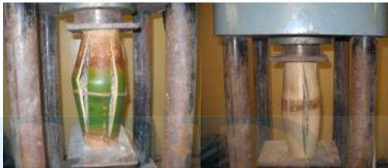
Fig. 3.4 (a) Reinforced Fresh Bamboo Under Compressive Test
