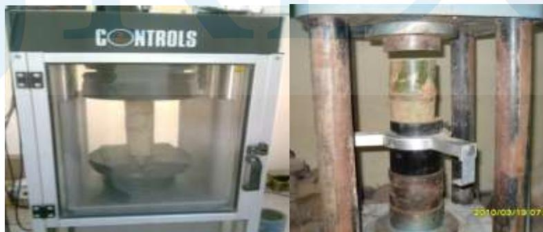
Fig. 3.4 (c) Dried Non-Reinforcement Bamboo Under Compressive Test
