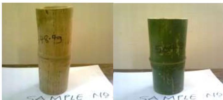
Fig.3.3. (c) Dried Bamboo Specimen without reinforcement
