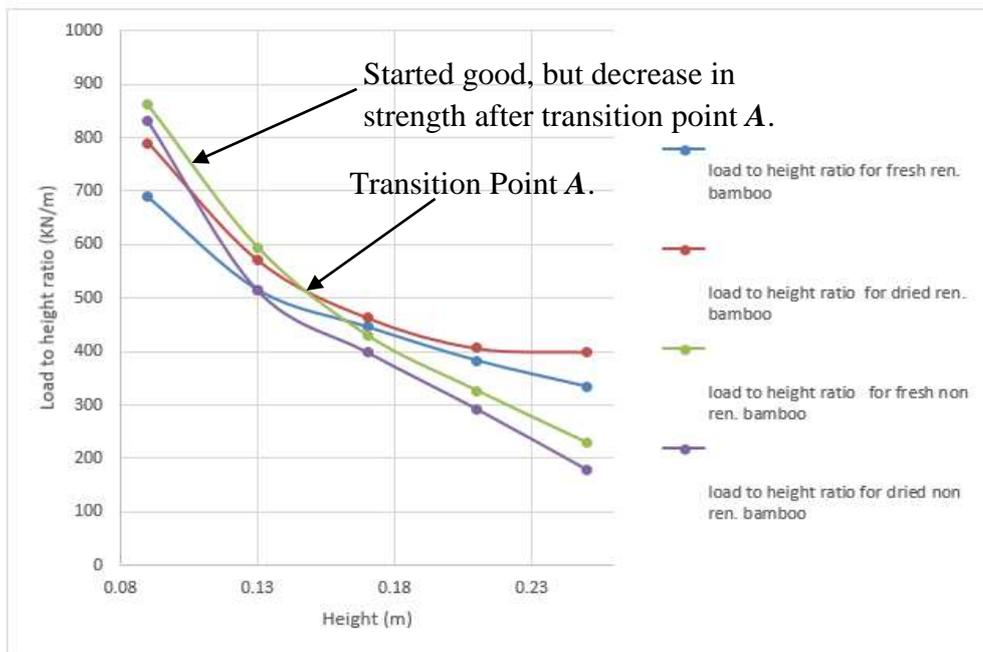
Fig. 3.8 Load to Height Ratio VS Height
