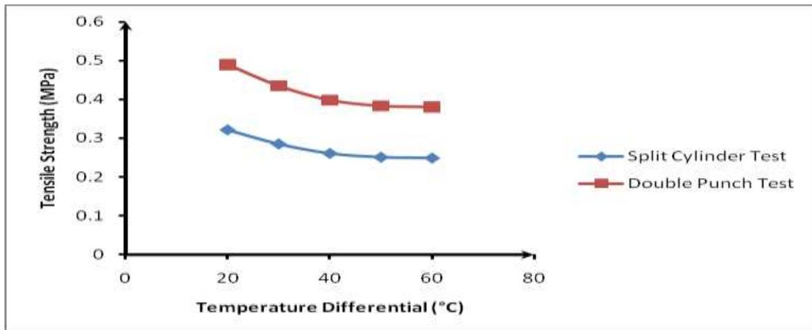
**Figure 1:** Tensile Strength Variation with Temperature Changes for Light Traffic
