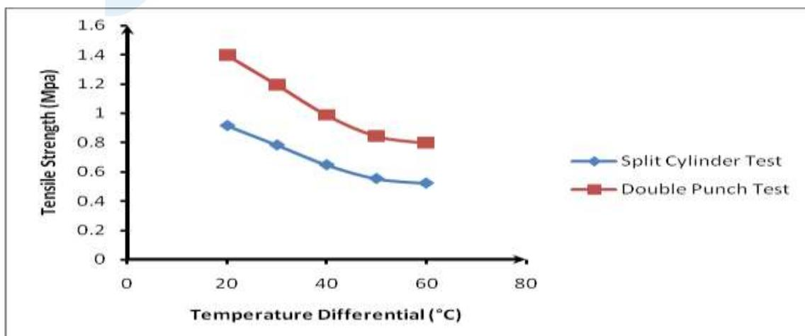
**Figure 3:** Tensile Strength Variation with Temperature Changes for Heavy Traffic
