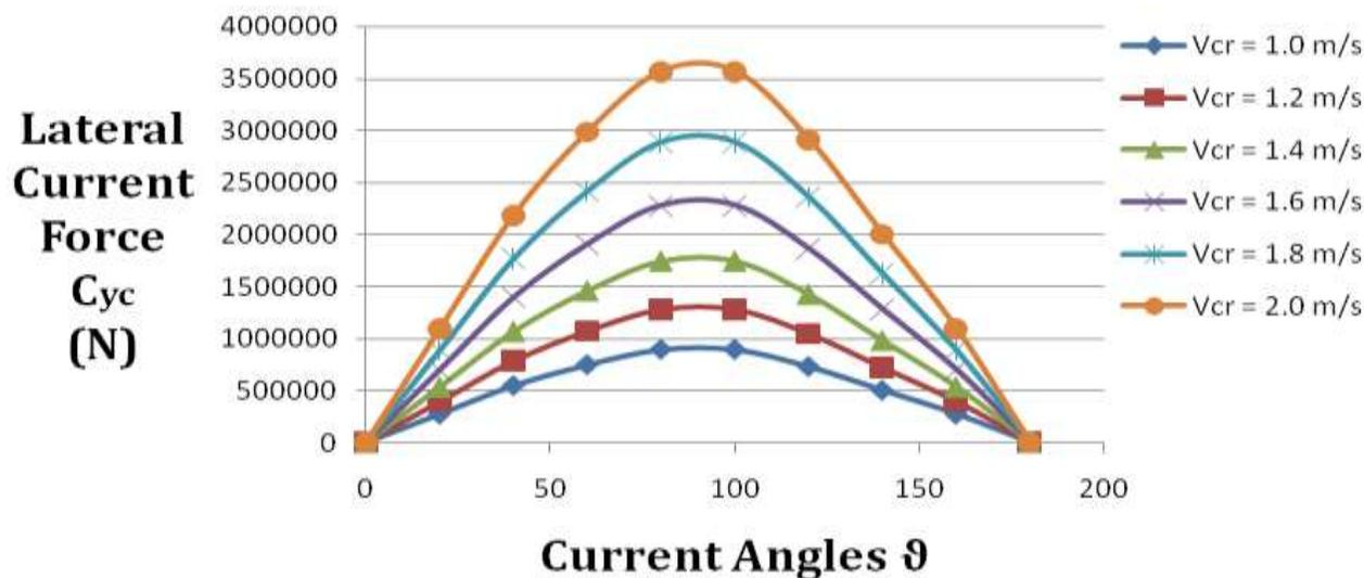
**Fig. E.2:** Lateral Current Force Coefficients versus angle of attack
