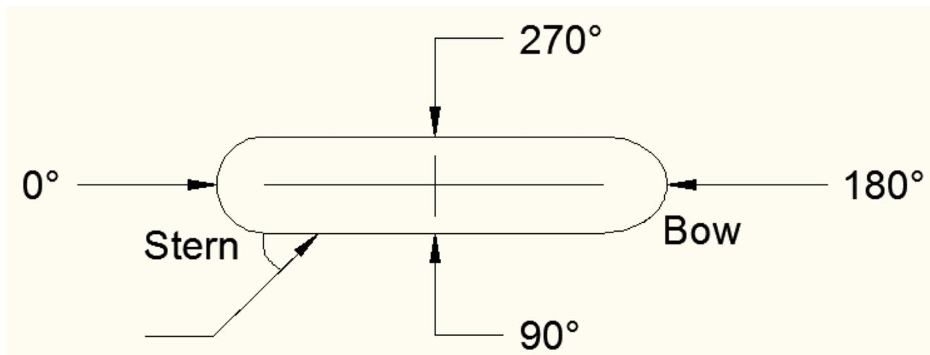
**Fig. 3:** Direction of wave heading/current attack angle
