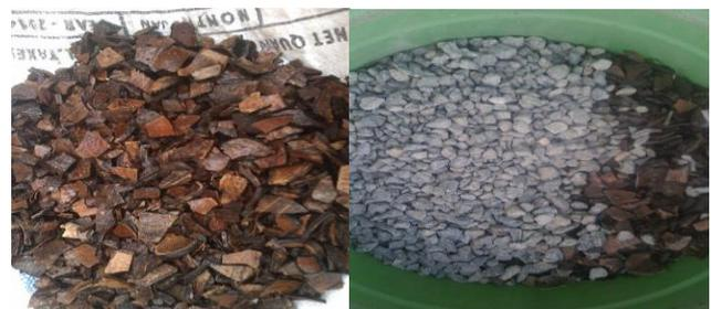
Fig.1 Sizes of coconut shell aggregate and normal aggregate
