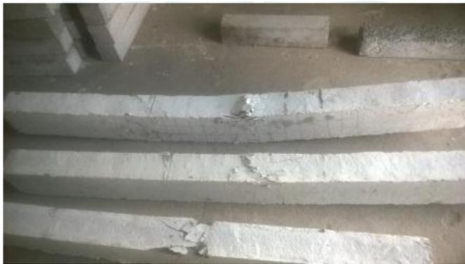
2. In the proportion of 10% fly ash content and 0.3% polypropylene fibre, the strength is maximum compared to the other proportions.
