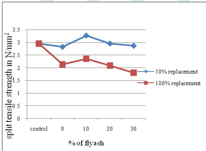
GRAPH-7 SPLIT TENSILE STRENGTH OF THE CYLINDERS AT 56 DAYS (COMPARISON OF COCONUT SHELL REPLACEMENT 50% AND 100%)
