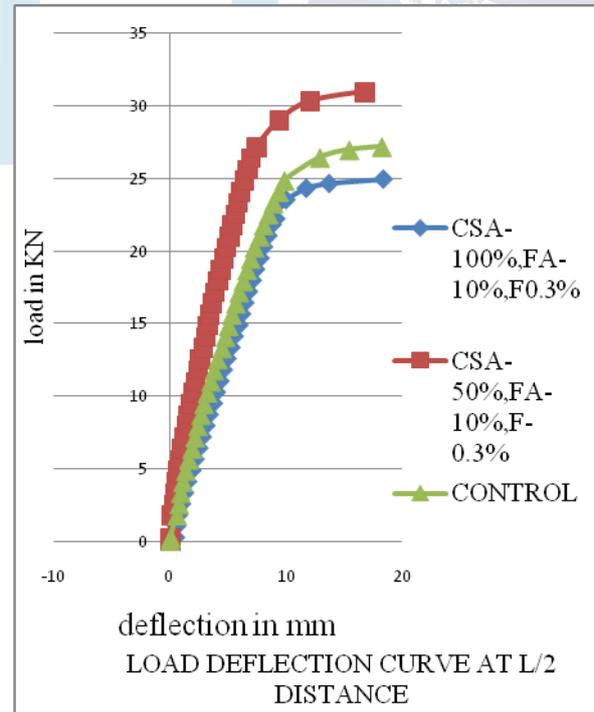
When comparing the load carrying capacity, the beam CSA-50%,FA-10%,F-0.3% gives higher ultimate load carrying capacity than the other beams. CSA-100%,FA-10%,F-0.3% having the maximum deflection.
