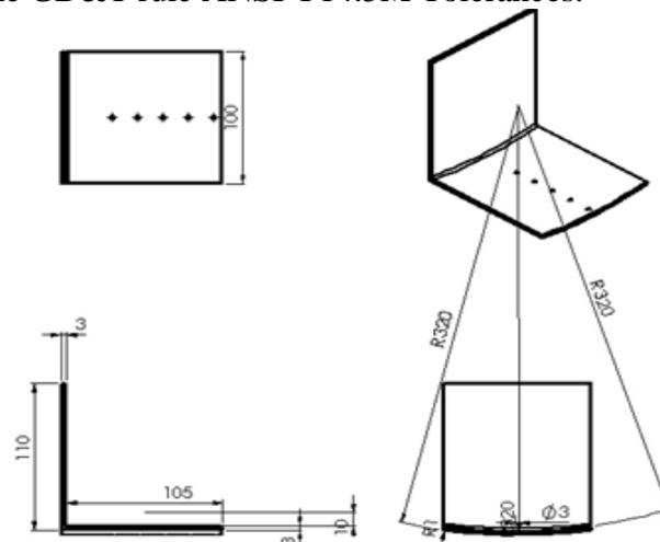
Fig 8: Dimensions of the limb mechanism.
