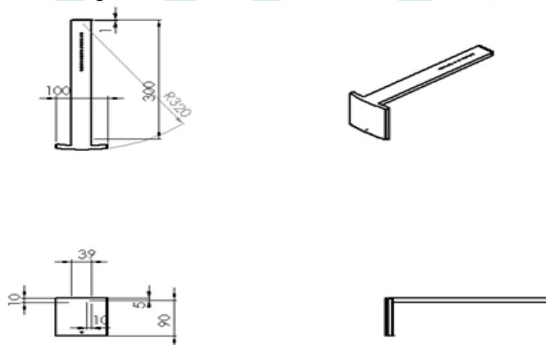
Fig 10: Dimensions of the top arm.
