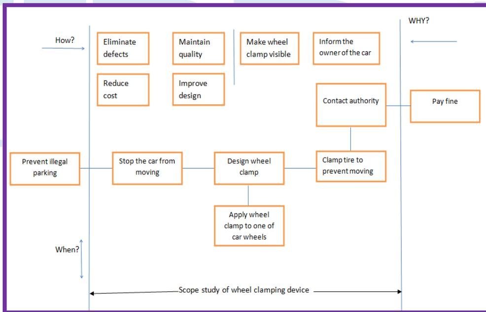
Fig 6: The FAST sketch for the case in hand.
