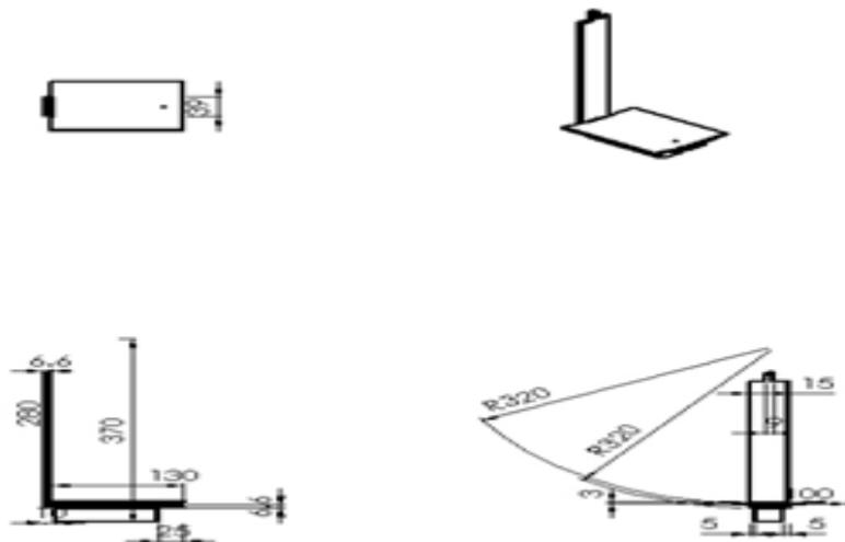
Fig 9: Dimensions of the bottom limb.
