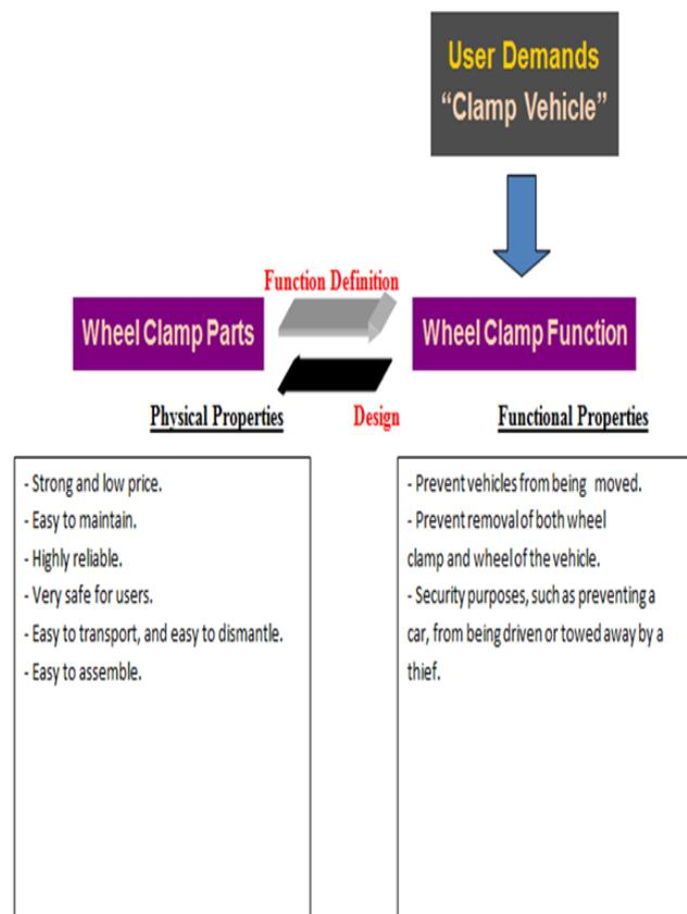
Fig 7: Functions and physical properties of the device.
