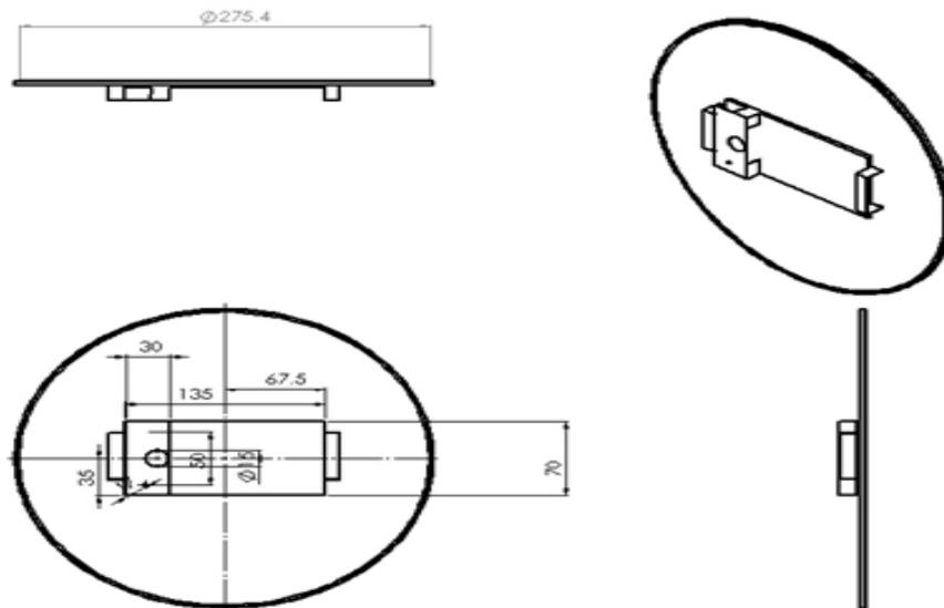
Fig 11: Dimensions of the latch shield.
