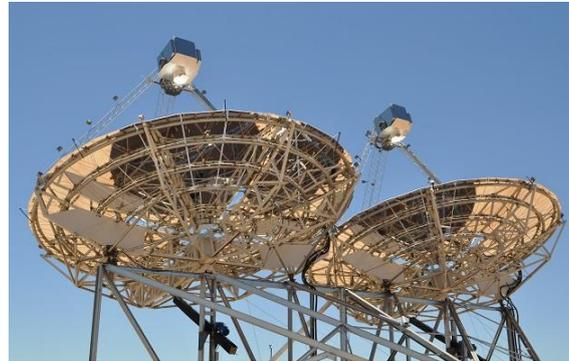
Figure4:- Cavity Receiver of solar Paraboloid Dish (source: - NREL)
