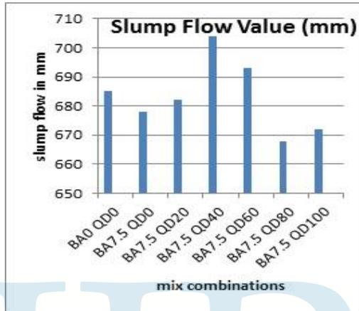
Figure4.1 Slump Flow Test Values
