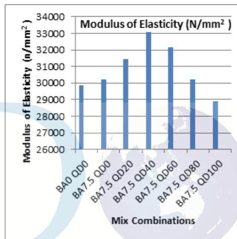
TABLE 4.8 DENSITY AND MODULUS OF ELASTICITY ALL CONCRETE MIXES
