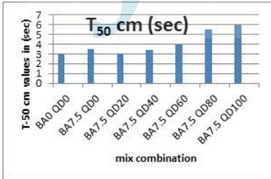
Figure 4.2 T<sub>50</sub> cm Slump Test Values
