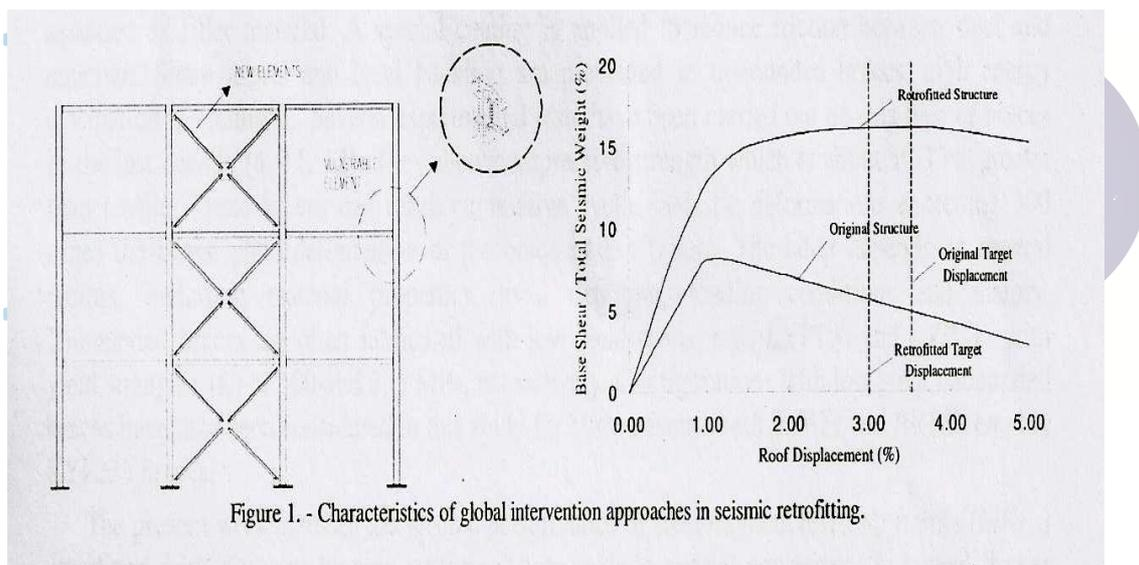
**Figure 2** Characteristics of global invention in seismic retrofitting
