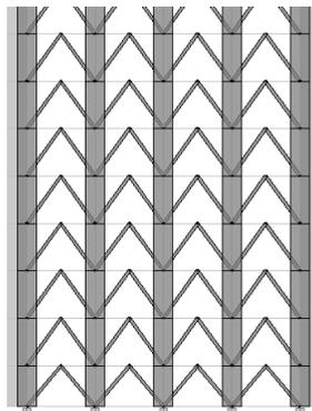
Fig-1 Showing inverted v bracings
