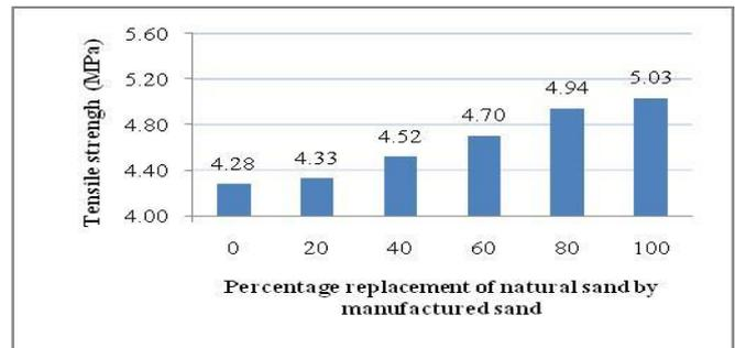
Fig 2: Variation in split tensile strength of concrete
