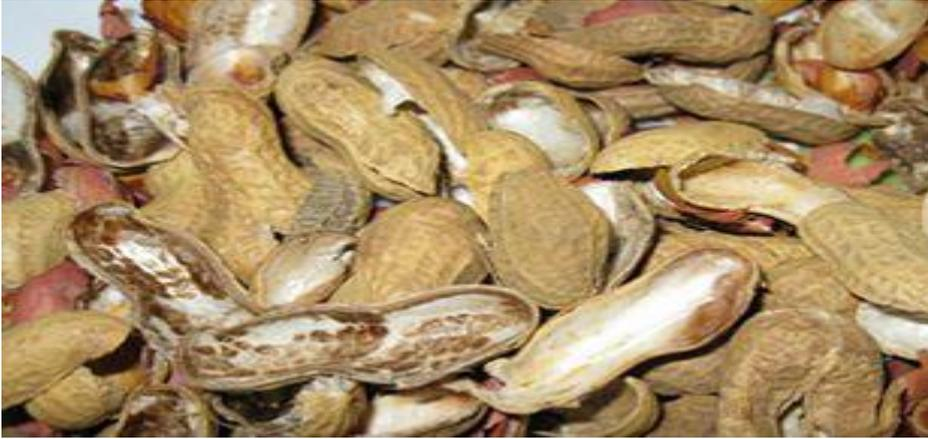
Ground nut shell ash was partially used cement in concrete. Thus, the possible use of agriculture waste (such as Ground nut shell ash-GSA) will considerably reduce the cost of construction and as well as reduce or eliminate the environmental hazards caused by such waste.
