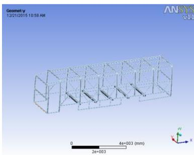
4.1 Geometry of the Bus Body Super Structure
