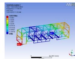
4.31: Model 2: Max deflection is 1.8431mm when the frequency is 7.1149Hz
