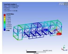
4.33: Mode 4: Max deflection is 2.81590 mm when the frequency is 13.996 Hz
