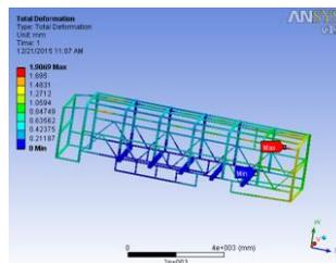
4.17: Max deformation is 1.9069 mm at 10500 N load applied on cant rail
