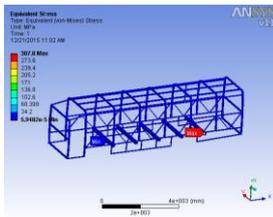
4.26: Equivalent stress developed is 307.8 Mpa at 10500 N load applied On cant rail
