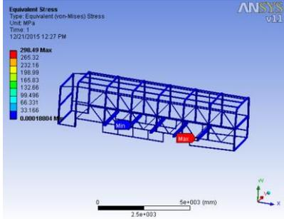
4.8 Equivalent stress developed is 752.85 Mpa at 49275 N load on waist rail
