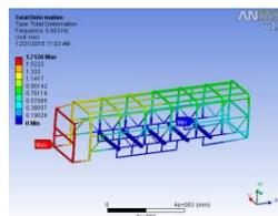
4.30: Model 1: Max deflection is 1.726mm when the frequency is 5.903Hz
