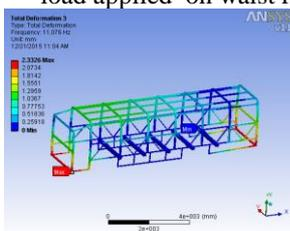
4.32: Mode 3: Max deflection is 2.3326 mm when the frequency is 11.076 Hz
