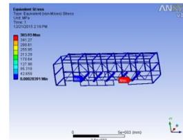
4.28: Equivalent stress developed is 822.02 Mpa at 49275 N load applied On waist rail
