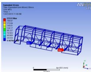
4.16: Equivalent stress developed is 223.51 Mpa at 10500 N load applied On cant rail
