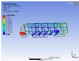
4.29: Max deformation is 2.7925 mm at 49275N load applied on waist rail
