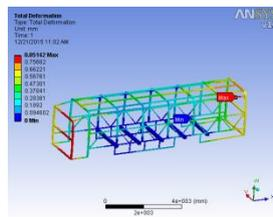
4.27: Max deformation is 0.85142 mm when load is 10500N applied on cat rail
