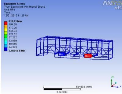
4.6 Equivalent stress developed is 218.91 Mpa at 10500 N load applied On cant rail
