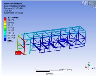
4.34: Mode 5: Max deflection is 3.2145 mm when the frequency is 19.214 Hz
