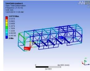
4.35: Mode 6: Max deflection is 3.9733 mm when the frequency is 21.53 Hz
