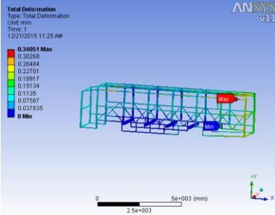
4.7 Max deformation is 0.34051mm when 10500N load is applied on cant rail
