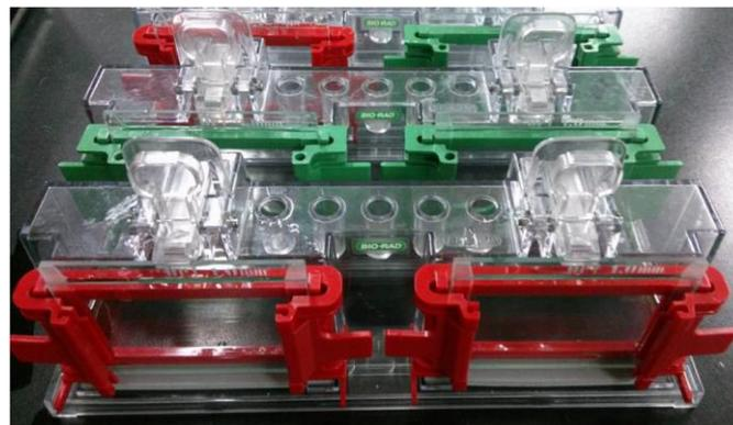
**Figure 3. Fixing the bottom-sealed glass plates to the frames for casting**
