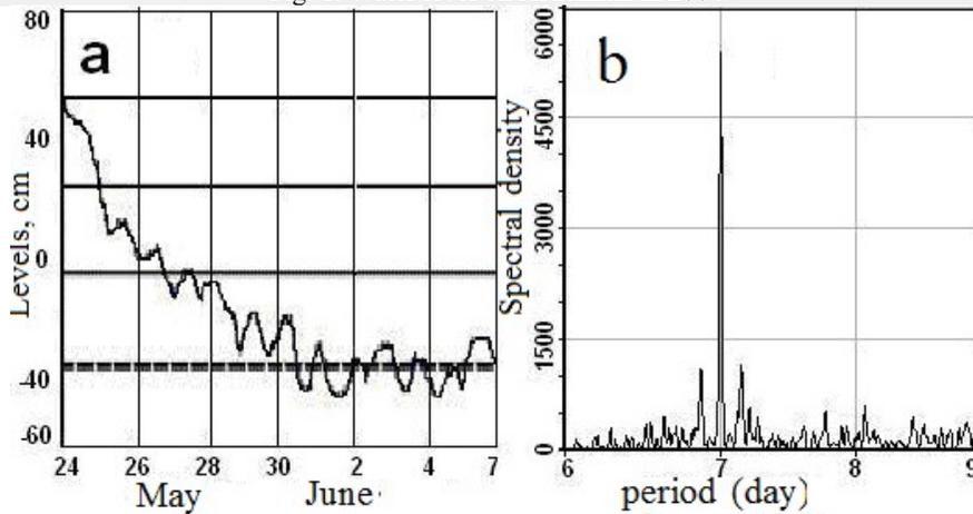
Fig. 2. Recording of the level on the railway station Astrakhan from 24.05 to 07.06.1992 (a) [14] spectral density of water level fluctuations on the Lower Volga in 1992-2003 (b) [8].
